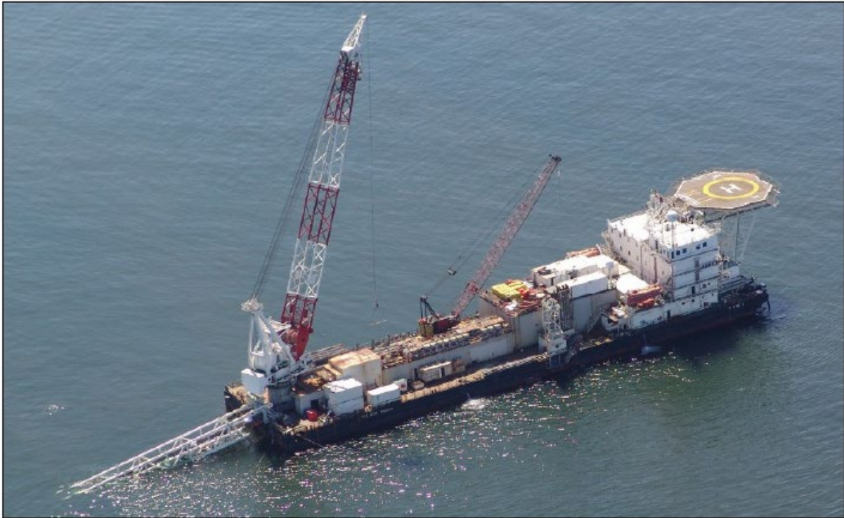
Figure 2-7 Example of pipelaying vessel (nearshore pipelay barge)
