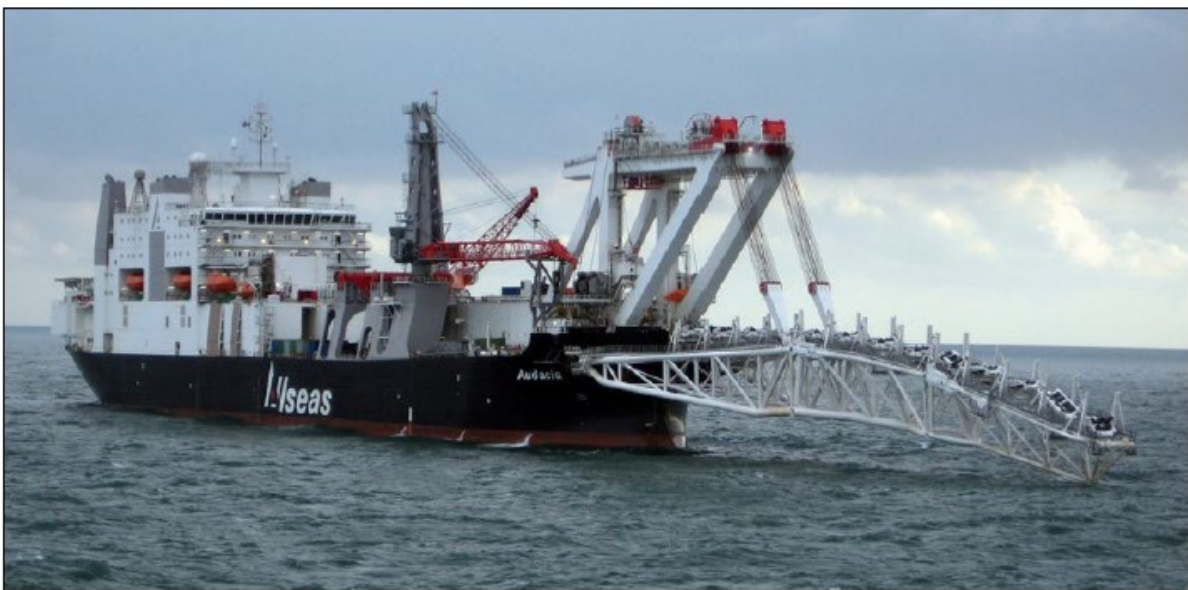
Figure 2-6 Example of pipelaying vessel (deep water vessel)
